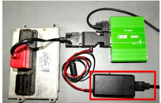
There are two methods, read out the ACM in mounted position also. The ACM can be directly supplied with power when the connection no longer works at the OBD connector. Both methods can cause problems, so it is better, to dismount the ACM and read at a desk or a workbench. An additional advantage occurs if the ACM can be kept if possible, since data protection and traceability is ensured (evidence by forensic chain).
